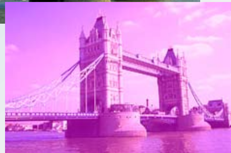
Dye fading in a traditional photographic color print usually results in an overall pinkish cast (seen in the lower image), due to the fact that the cyan and yellow dyes fade faster than the magenta dye.
